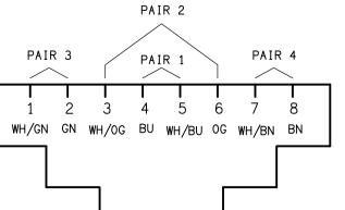
**SCHEMATIC RJ45 PINOUT CONFIGURATION** NOT TO SCALE
