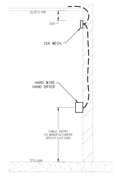
**DETAIL** HAND DRYER CONNECTION NOT TO SCALE
